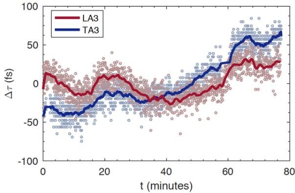
Figure 6: Change in delay between North and South beams measured in both LA3 and TA3 against time. The drifts and oscillations measured by the two diagnostics are strongly correlated, but the TA3 diagnostic experiences an additional slow drift of around 80 fs over 80 minutes.
