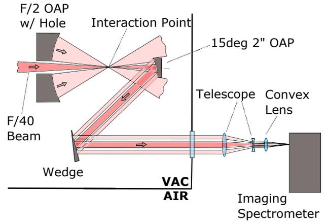
Figure 1: Experimental layout for the off-shot timing diagnostic, located post-IP in TA3.
