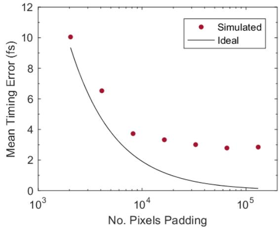
Figure 4: Simulated measurement error against pixels of zero-padding for a 600 lines per mm grating at 800 nm. Increasing the number of points in the frequency grid improves the resolution of the measurement towards zero, but the precision approaches a finite limit.
