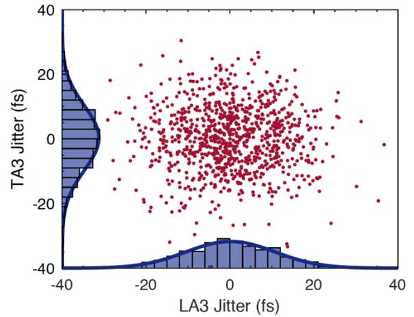
Figure 7: Comparison between jitters from LA3 and TA3 measurements, matched shot to shot. There is no correlation, implying that the jitters are independent random measurement errors with standard deviations of  $(10.6 \pm 0.7)$  fs and  $(10.0 \pm 0.6)$  fs respectively.
