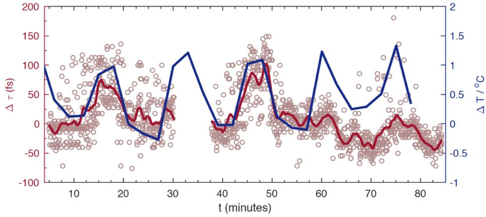
Figure 5: Change in delay between North and South beams measured in TA3 (moving average in red line) against time compared to temperature measured in LA3 (blue line). Variation in delay on the scale of 100 fs correlates strongly with 1 degree changes in temperature which are periodic over around 15 minutes.
