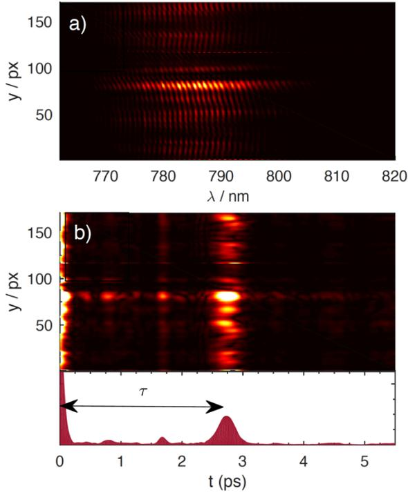
Figure 2: a) An example spectrum showing timing fringes, measured in TA3, from the interference of the North and South Beams separated in time. b) The Fourier transform of this spectrum shows the fringe frequency, which corresponds to a time delay  $\Delta t = (2.74 \pm 0.01)$  ps.
