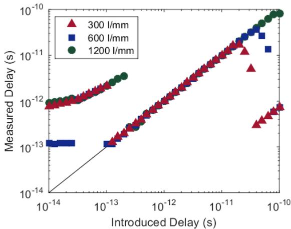
Figure 3: Simulations of measured delay against introduced delay for a range of different dispersions, and hence spectrometer bandwidths. More dispersive gratings are effective at higher delays, up to around 0.1 ns, but fail sooner at small delays of 100s of fs, where the sideband can no longer be resolved from the DC peak.
